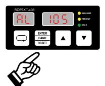
Invalid error messages may appear when the controller is switched off owing to the undefined operating state. This must be taken into account when they are evaluated by the higher-level controller (e.g. a PLC) in order to avoid false alarms.
