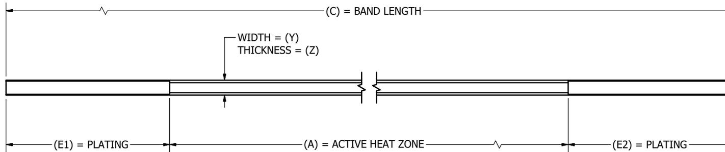
STEP #1 ... ENTER REQUIRED HEAT SEAL BAND/WIRE DIMENSIONS:
