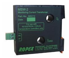
In certain applications with RESISTRON or CIRUS temperature controllers, it is necessary to detect shortcircuits between the heatsealing band and ground or the housing. In this case, the control system must be immediately switched off. The MSW-2 monitoring current transformer can be used for this purpose.
